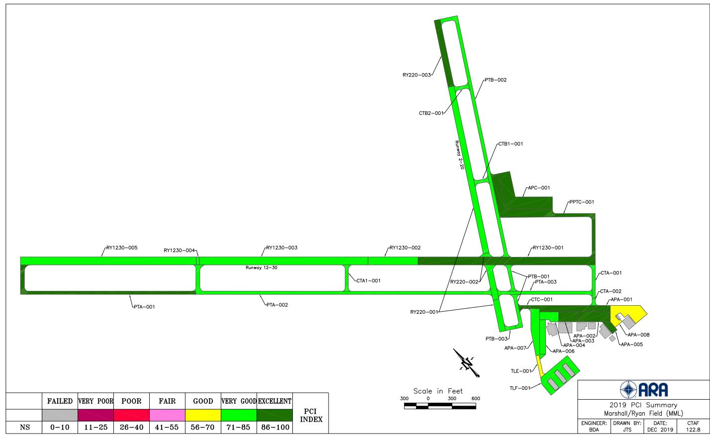
Figure 4. 2019 Pavement Condition Index Rating at Southwest Minnesota Regional Airport — Marshall/Ryan Field (MML).
