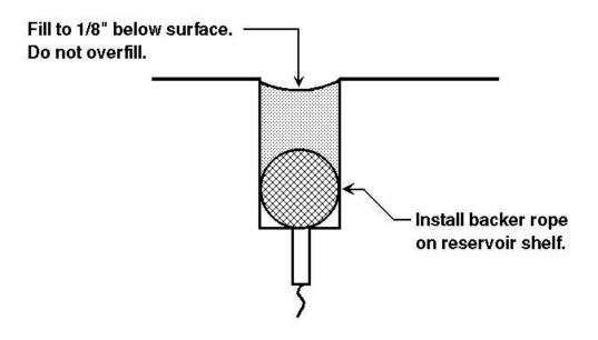
Figure G.6. PCC joint/crack repair.
