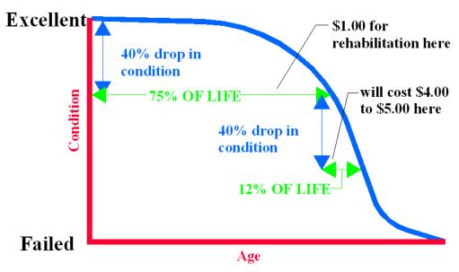
Figure 1. Pavement condition life cycle.
