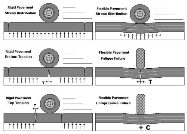
Figure G.1. Pavement failure.
